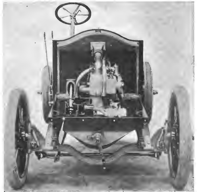
FRONT VIEW, SHOWING ACCESSIBILITY OF ENGINE.
